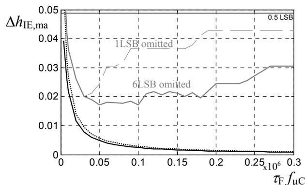
Fig. 1. Dependency of maximal IE error  $\Delta h_{IE,max}$  on time constant of RC-filter  $\tau_F$ . Theoretical/simulation error without quantization - black solid line/dots; Simulation error including quantization if 6 or 1 LSB omitted at both ends of scale gray lines
