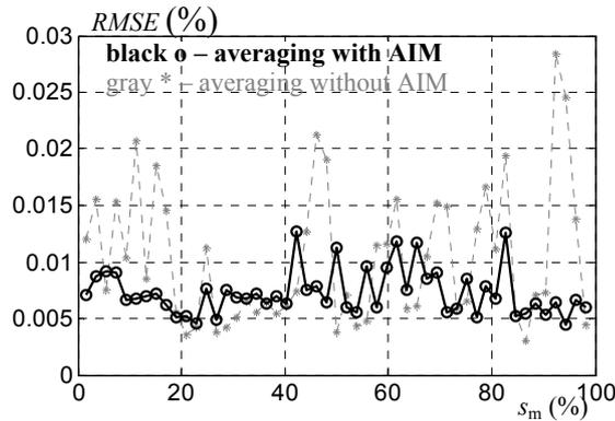
Fig. 4. RMSE of ADC with dithering before and after correction with AIM
