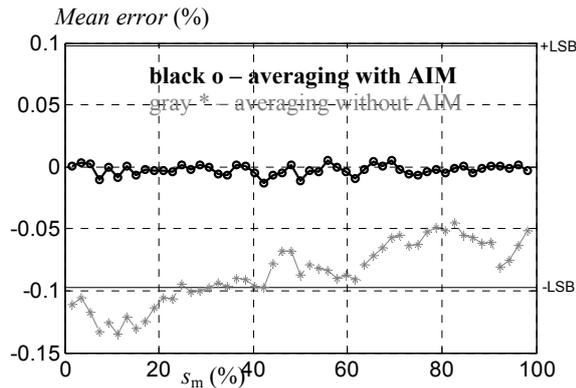
Fig. 3. Mean error of ADC with dithering before and after correction with AIM
