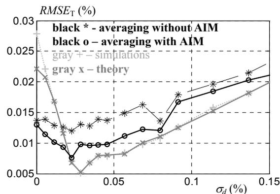
Fig. 2. Dependency of the total RMSE of ADC with averaging on standard deviation of dither before and after correction with AIM
