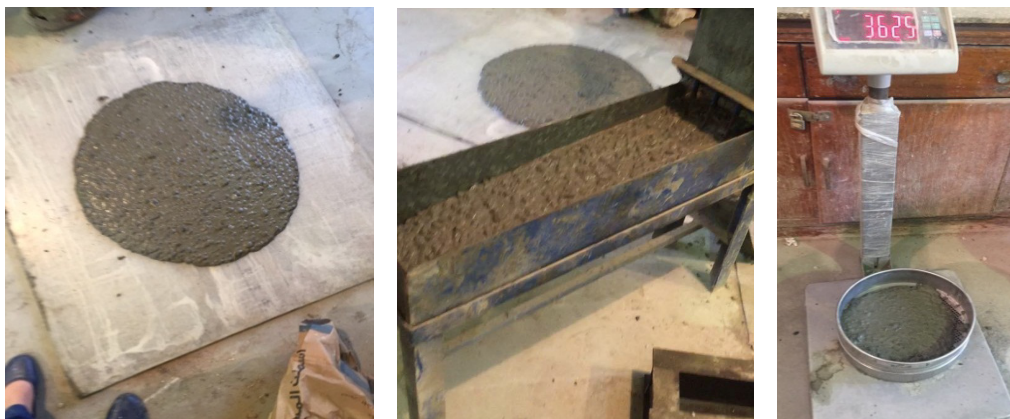
Fig. 4. Fresh concrete tests: slump flow, L-Box and segregation resistance tests
