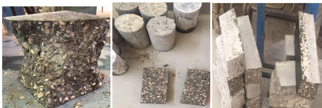
Fig. 7. Concrete cubes, cylinders and prisms after testing
