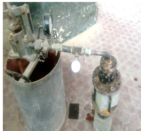
Fig. 6. Water permeability equipment
