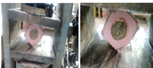
Fig. 8. Specimen extracted from permeability equipment
