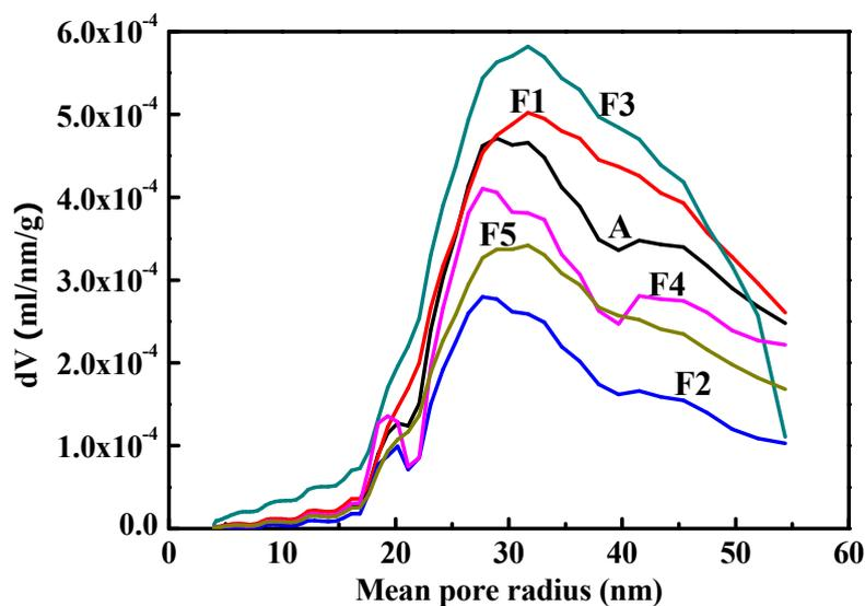
Fig. 4. Pore- Size Distribution Curves of GO- Cement Composites
