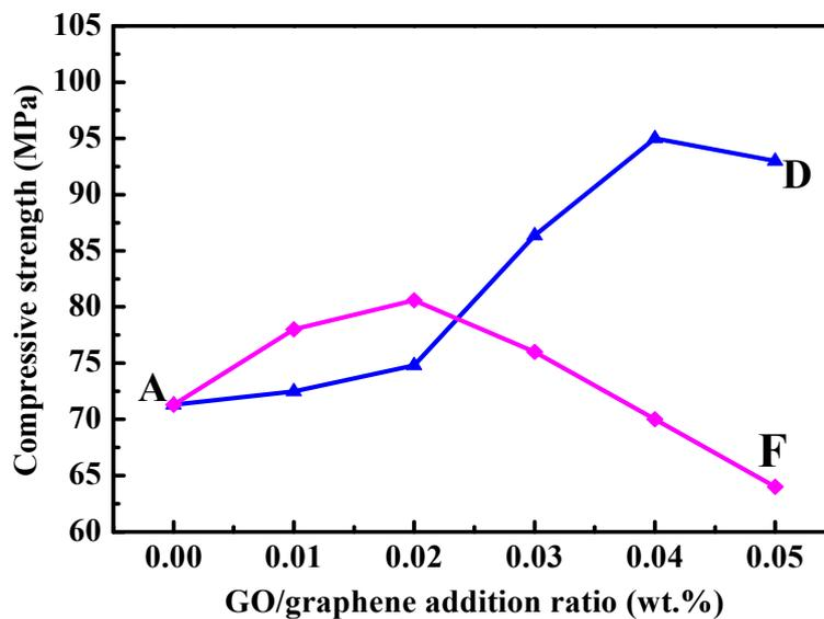
Fig. 2. Compressive strength of the hardened GO/GNSs - OPC composites
