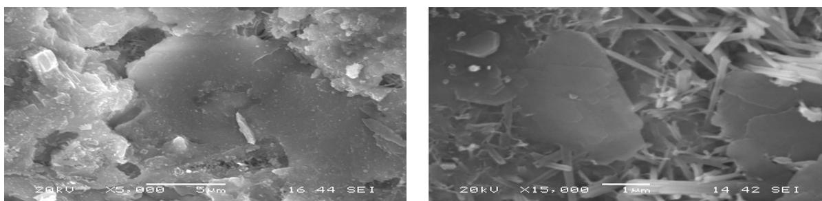
Fig. 9. SEM images of cement paste modified with GO sheets
