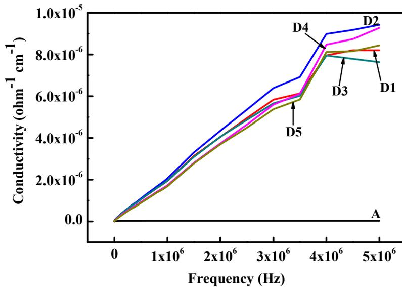
Fig. 11. Electrical conductivity of graphene - cement composites
