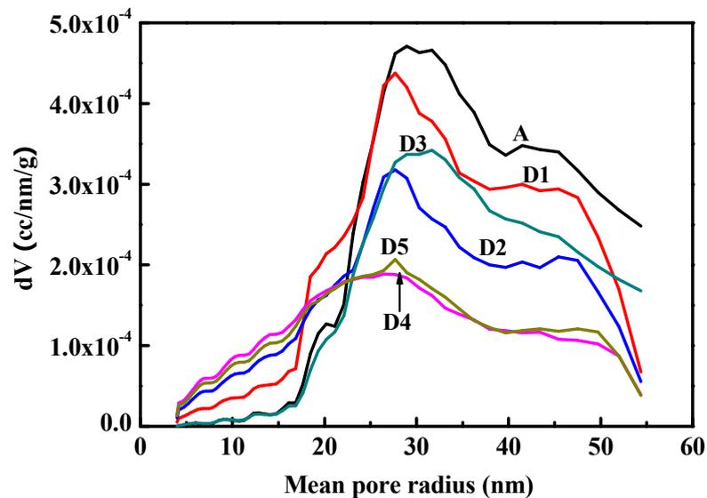
Fig. 3. Pore- size distribution curves of graphene-cement composites
