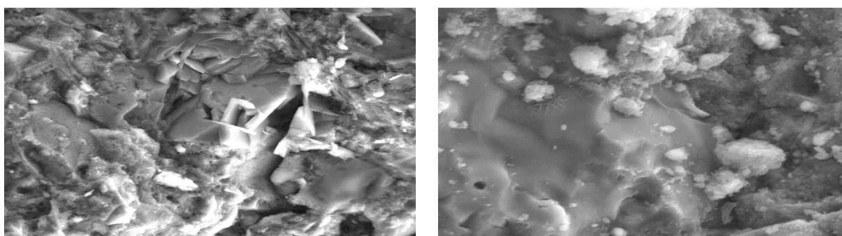
Fig. 8. SEM images of cement paste modified with graphene sheets.
