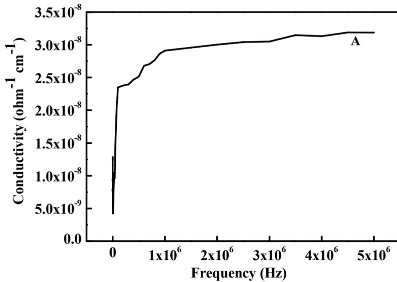
Fig. 10. Electrical conductivity of neat cement paste
