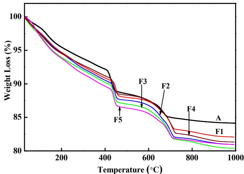
Fig. 6. TGA Thermograms of GO – Cement Composites
