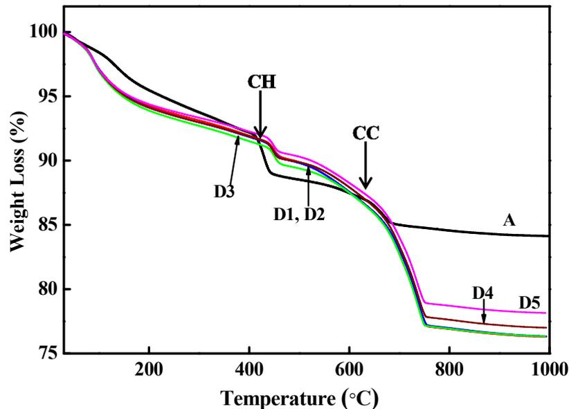
Fig. 5. The TGA thermograms of graphene– cement composites
