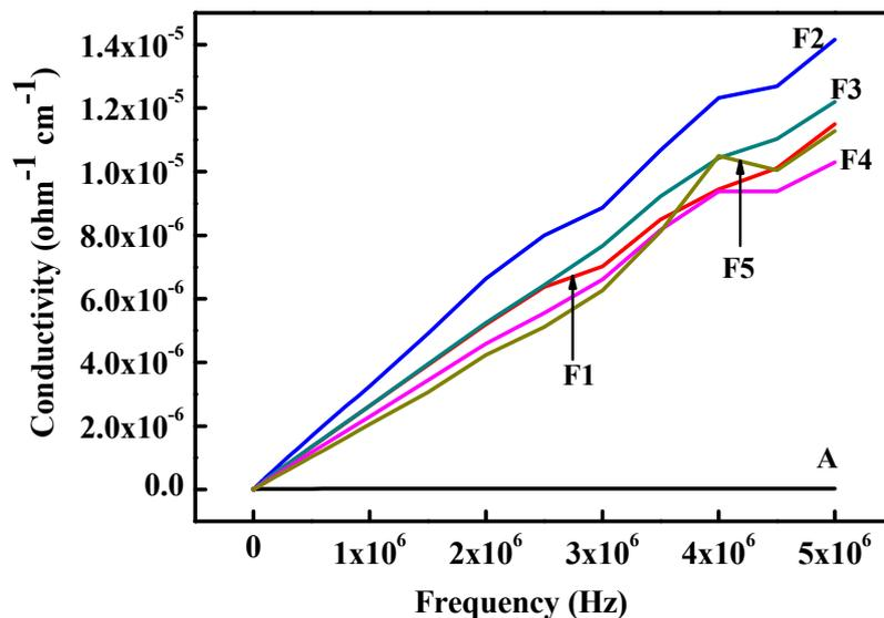
Fig. 12. Electrical Conductivity of GO- Cement Composites
